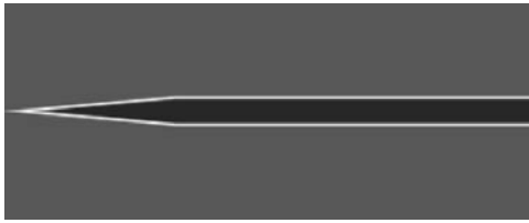
Figure 2. The initial configuration for the simulation of a needle tip just touching the surface, with the centre of the domain wall highlighted (in reality the domain wall is much wider).
